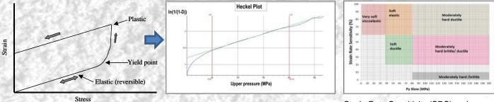
Particle Deformation – the test compresses the API or excipient until it yields.
