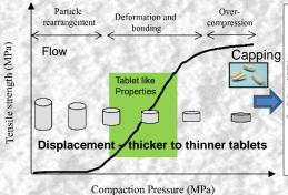
Large increase in strength with small change in force – process may be difficult to control be difficult to control
