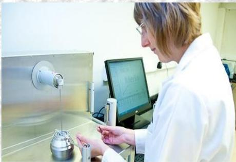
A choice of the loading forces can be applied to mimic the powder in different sized containers i.e. Large normal load for large hopper
