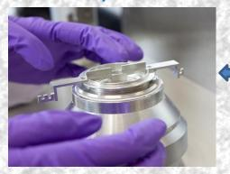
A choice of the loading forces can be applied to mimic the powder in different sized containers i.e. Large normal load for large hopper
