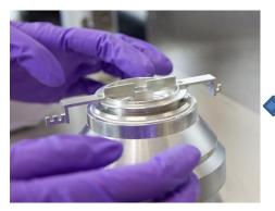
A choice of the loading forces can be applied to mimic the powder in different sized containers i.e . Large normal load for large hopper
